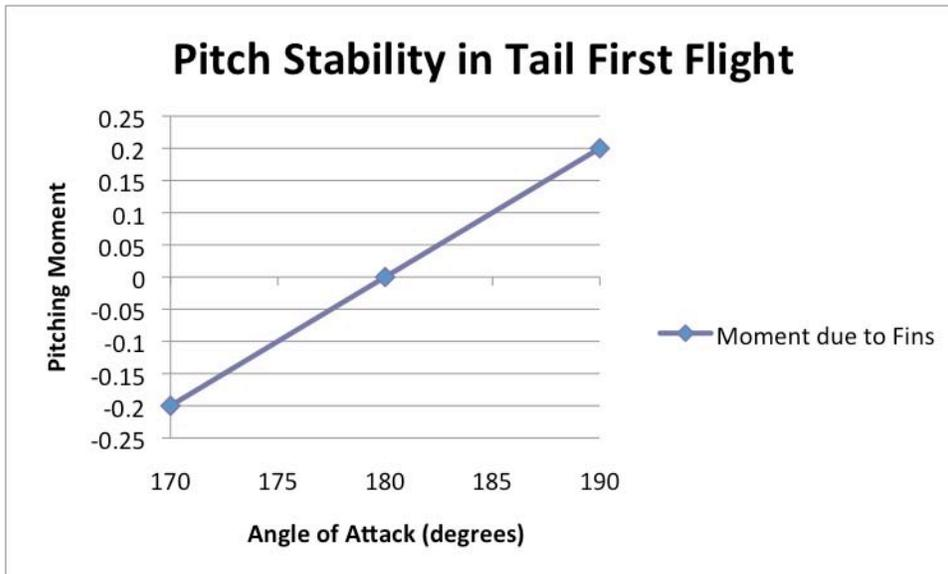
**Figure 8 Moment vs Angle of Attack for a normal stable rocket in tail first flight. The positive slope of the curve implies that the rocket is not stable in this orientation.**
