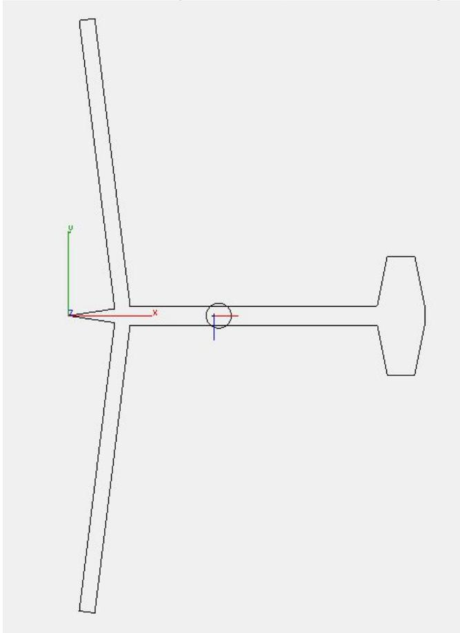
**Figure 5 Center of Lateral Area drawing for large rotor, with chord scaled to 50%. CLA is close to drop test CM**
