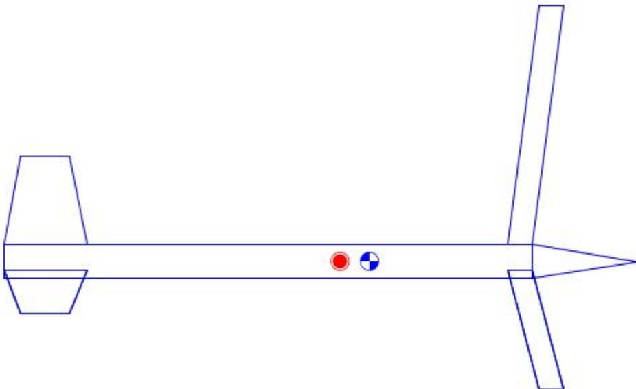
**Figure 2 Same model in Open Rocket, but rotated to tail first orientation. Same scale factor on rotor as above. Note that this case shows a slight nose first stability**
