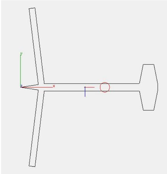
**Figure 6 CLA for small rotor, with the same scale factor as above. CLA is well ahead of CM indicating tail first stability**
