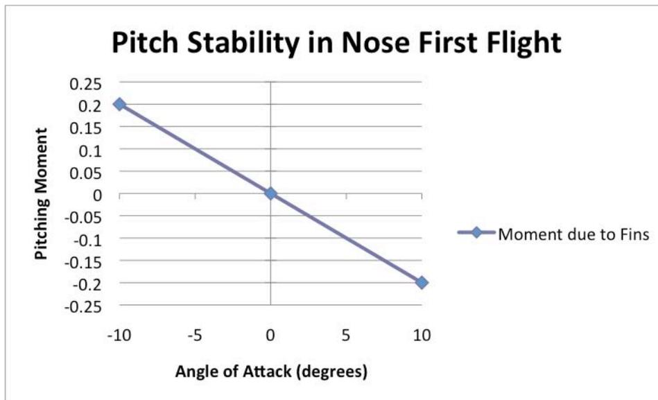
**Figure 7 Moment vs Angle of Attack for a conventional, stable rocket**
