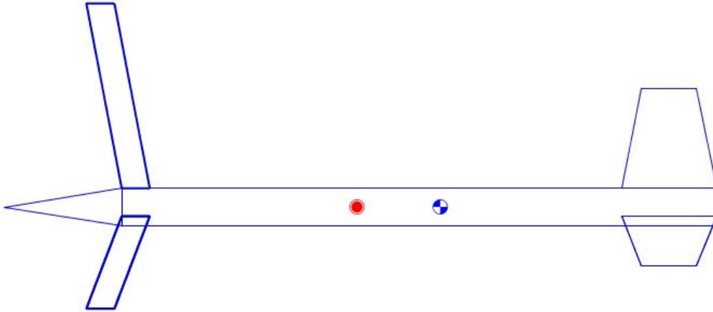
**Figure 3 small rotor nose first case, same scale factor as above. Note that this case shows strong tail first stability**
