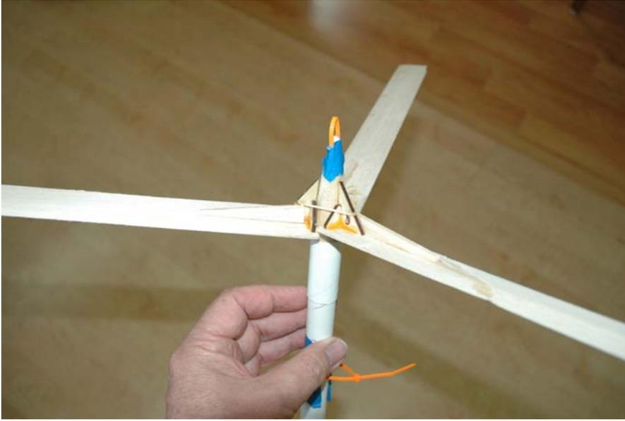
**Picture 4. Close up photo of a typical rotor hub assembly the pitch and cone angles were each set by a laser cut plywood piece, and the two pieces fit each other with laser cut notches to ensure consistent alignment. The rotor blade root was left square to mate precisely with the laser cut parts. After initial breakage, the balsa extension and kevlar wrap were added.**
