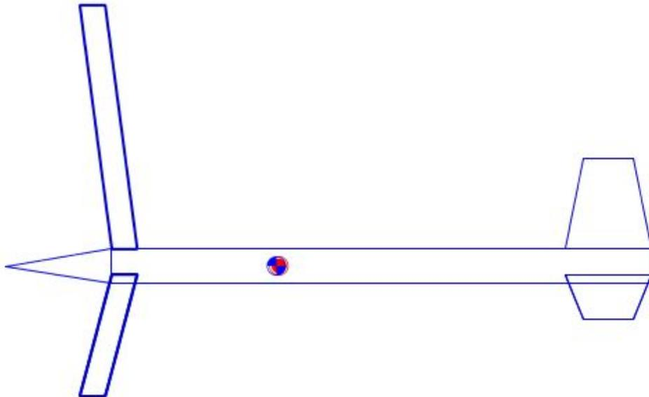
**Figure 1 Open Rocket nose first case, with scaled 12" radius rotor. Scale adjusted to put CP on CM**
