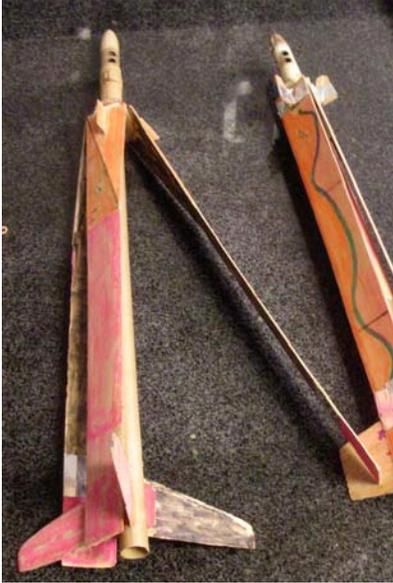
**Picture 1. An early model made by Coleman at left, showing evidence of fin fillets made of clay in attempt to cause tail-first descent.**
