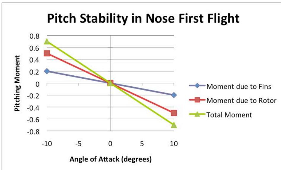
**Figure 9 The same rocket as before, but now with a rotor stability term added. In this case the fins and rotor are both stable, resulting in strong overall stability**
