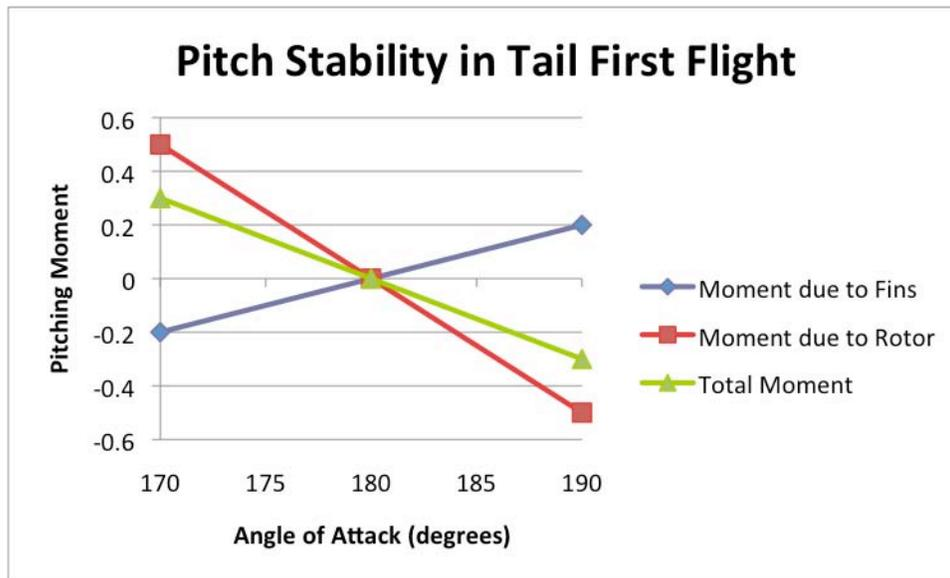
**Figure 10 The same rocket as above, but now in tail first flight. The fins result in instability, but the greater stability of the rotor results in net overall stability.**
