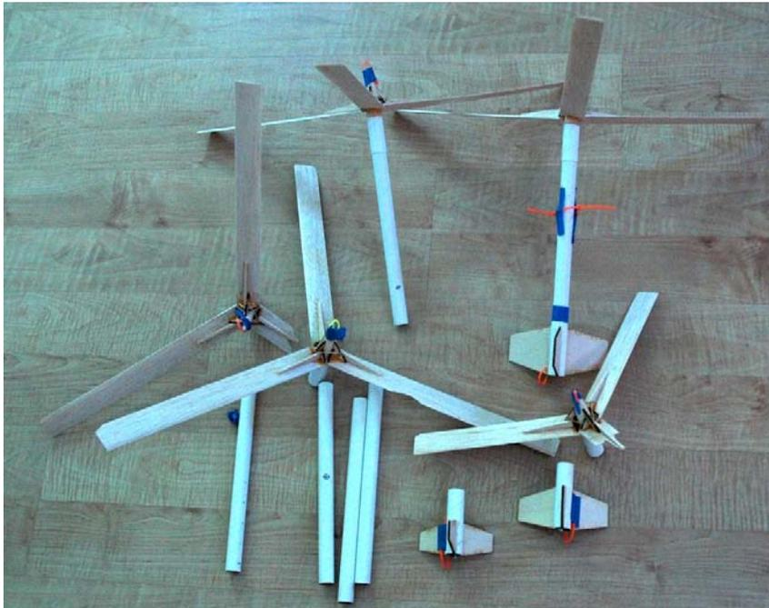
**Picture 3. Several of the modular model parts, one completed model at right. Pictures are post-testing, so some breaks are obvious.**
