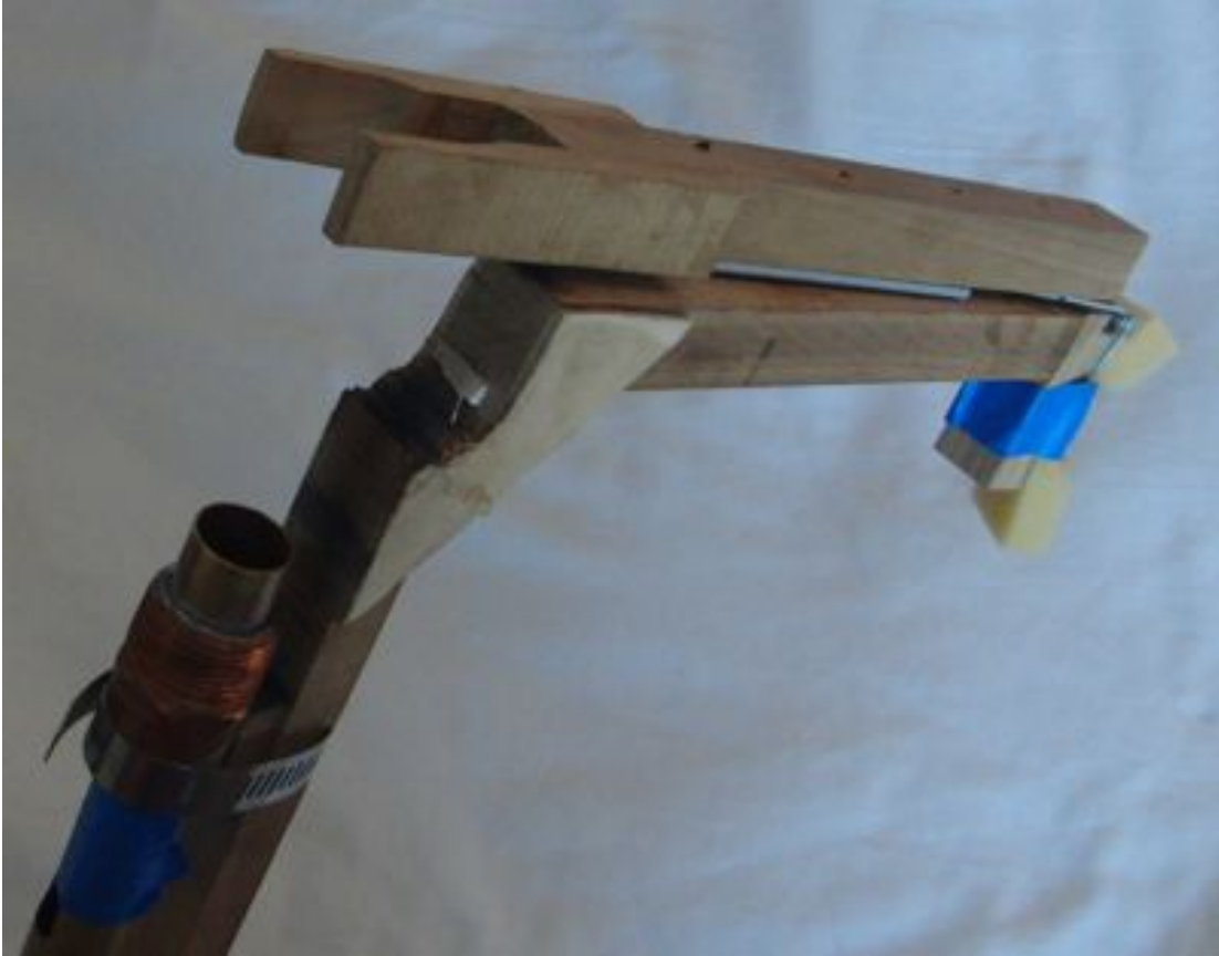
The top view showing the hold down arms that fit around the model and the steel attached to the swinging arm.
